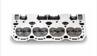
A Fast Burn Cylinder Head (combustion chamber)
