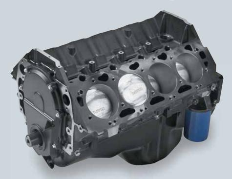
For those who want the sturdy foundation of the 454 HO as the starting point of a custom engine, this brand-new partial engine includes the forged crank, rods and pistons, as well as the balancer, oil pan and front cover. This partial engine does not included a camshaft, lifters, timing chain or cam sprocket. All parts necessary to complete the engine are available from your GMPP dealer. Use externally balanced flywheel for manual transmission applications.
