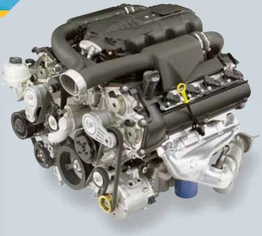
NOTE: Pulley, belt, power steering pump, air conditioning pump, starter, and alternator are not included with this engine.
