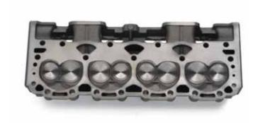
A, B Small and Large Port Vortec Bowtie Heads (combustion chamber)
