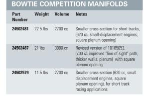
This chart illustrates the differences in some of the Bowtie Competition Manifolds. These single plane manifolds fit 18° cylinder heads and are designed with air gaps underneath the runners to insulate the intake charge from engine heat. Manifold flanges are 0.59" thick to promote a good gasket seal. An auxiliary water line boss at the rear of the casting improves water flow. Both P/N 24502481 and P/N 24502487 have square bore carburetor flange openings to match the spacers specified by NASCAR.
