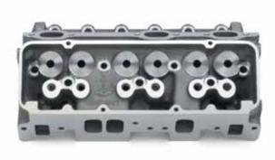
A 18° Aluminum Cylinder Head (top/intake)
