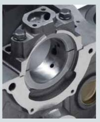
A Two-Bolt Rear Main (no seal adapter)
