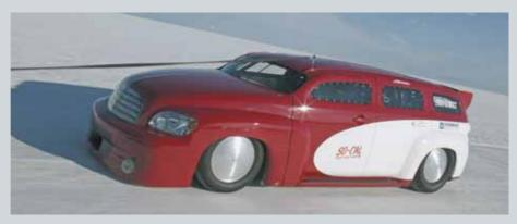
impressive, and assembled by four female engineering students. It went 140 mph in testing and is powered by 230 horsepower version of a turbocharged 16-valve Ecotec four cylinder.
